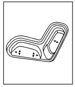
If the seats have power reclining seatbacks, use the vertical power seat control located on the outboard side of the seat.
